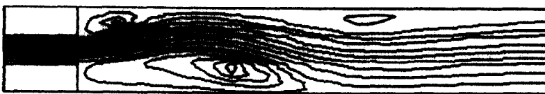
FIG. 7. Streamlines for two-dimensional symmetric sudden expansion duct flow at Re(H) = 250 and W/W_0 = 3 (numerical).
